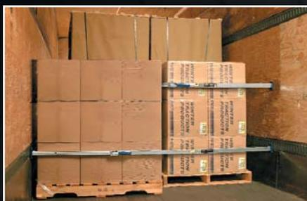
The SCC CargoBar™ can brace a whole load or just part of one.
